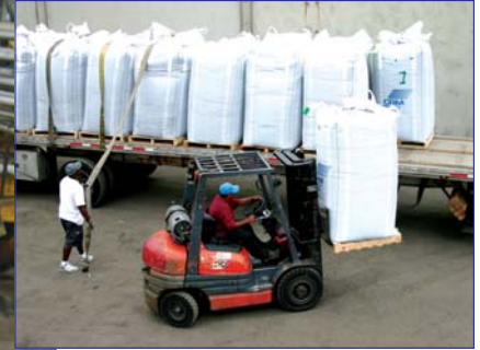
(Left & Above) Bagging crumb rubber into supersacks and then loading for delivery to rubberized asphalt contractors.
