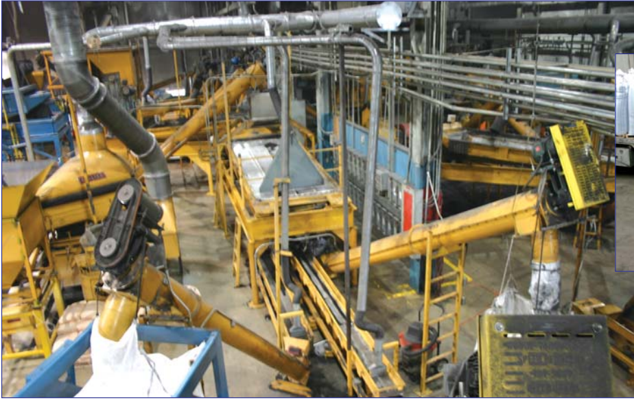
(Left & Above) Bagging crumb rubber into supersacks and then loading for delivery to rubberized asphalt contractors.
